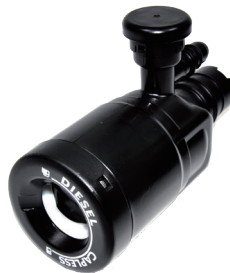
Capless & MFI Filler Neck - Prevents misfuelling into a diesel-powered vehicle - Convenient capless system enables drivers to release the door and immediately insert the fuel nozzle
