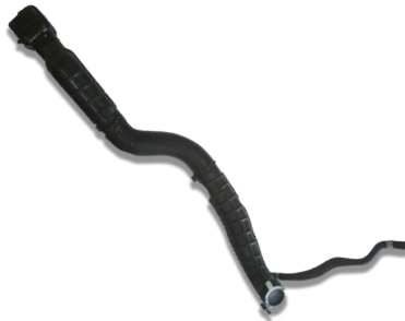
Air Intake Hose (*Part of Air Intake & Exhaust System) - Transfers the filtered air from the air cleaner to the throttle body or turbocharger - Absorbs vibrations generated during engine rolling
