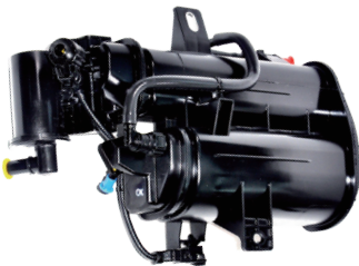
KLEV3 (South Korea) - Used in gasoline vehicles sold in Korea - Meets KLEV-3 environmental regulations enforced by the Ministry of Environment - Diurnal Bleed Emission Test: less than 350 mg/test
