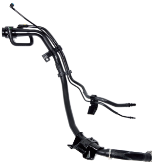
PA6+ Nano Filler Neck - Newly developed PA6+NANO material with excellent evaporative emissions barrier properties compared to the PA6 MONO-LAYER model
