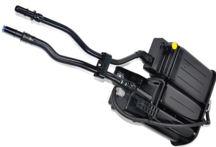
HEV LEV-3 / Tier-3 (North America) - Used in HEV vehicles sold in North America - Integration of ELCM parts for OBD2 fuel system evaporative leak diagnosis
